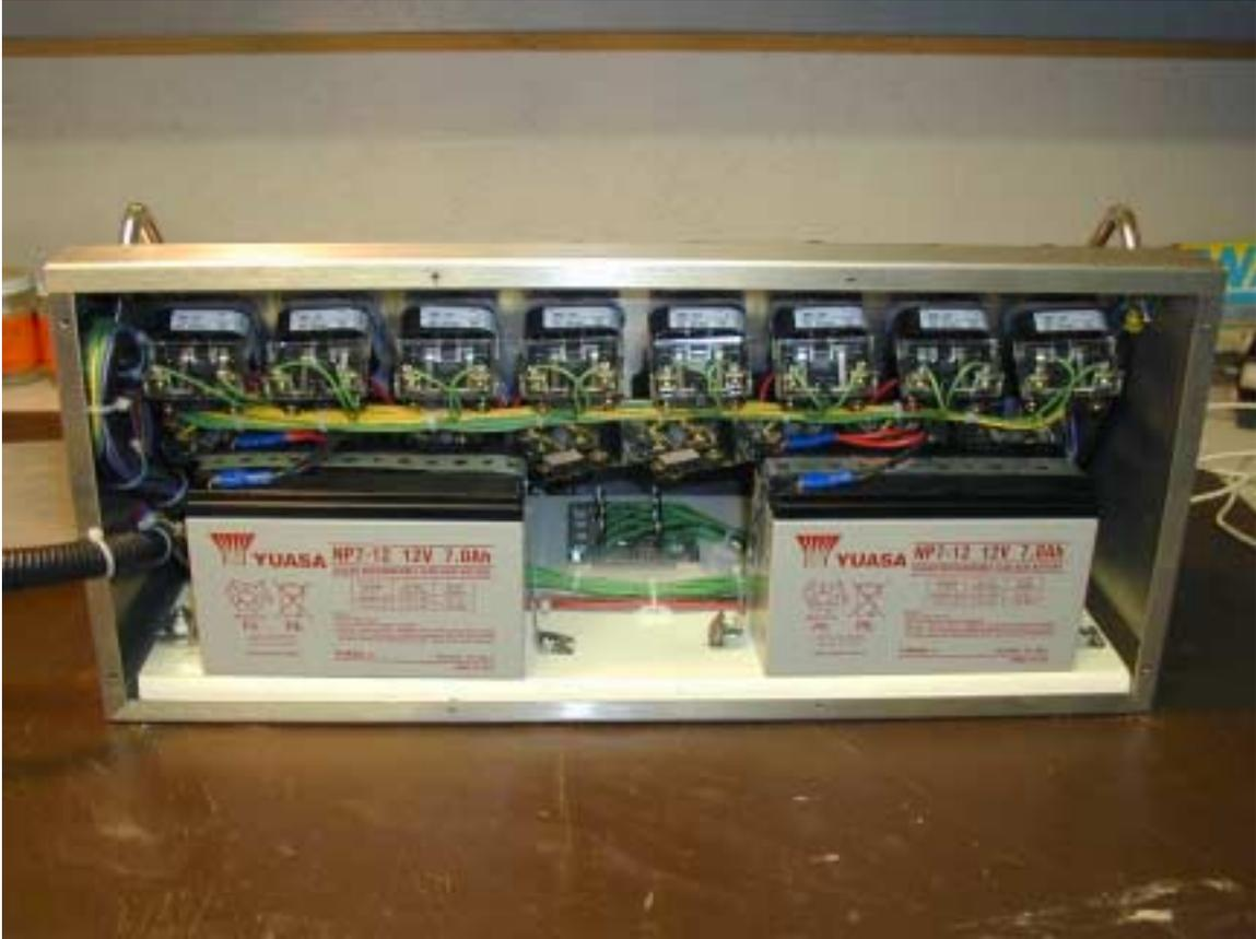
*Inside view of console showing batteries*
