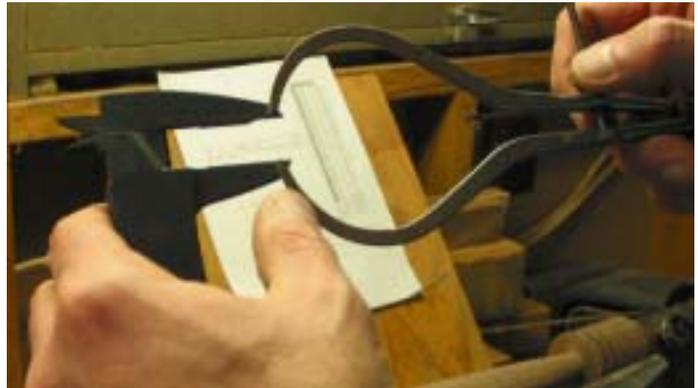
Figure 1. Setting the calipers
