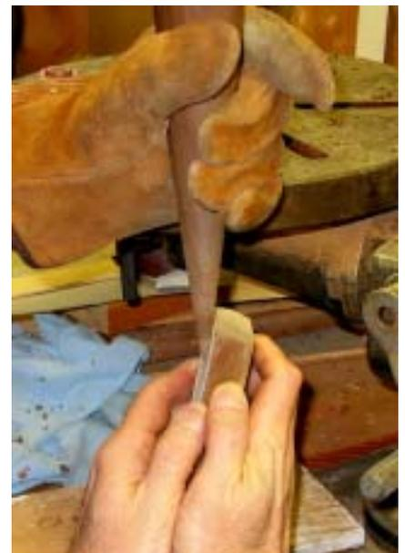
Figure 7. Sanding the tip using a drill press.
